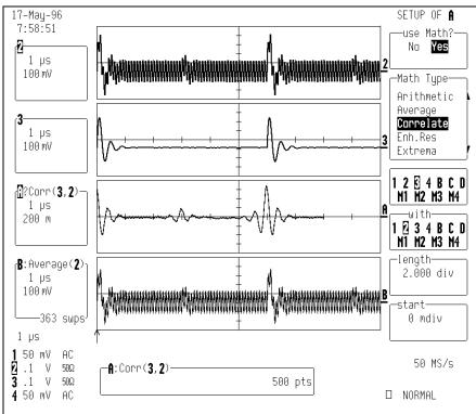
Figure 2 Cross correlation detects echo in interfering sine wave
